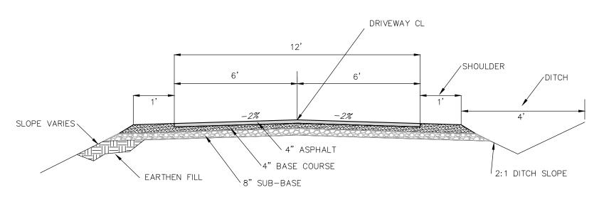
DRIVEWAY CROSS SECTION DETAIL: 12' DRIVEWAY W/ 1' SHOULDERS N.T.S.
