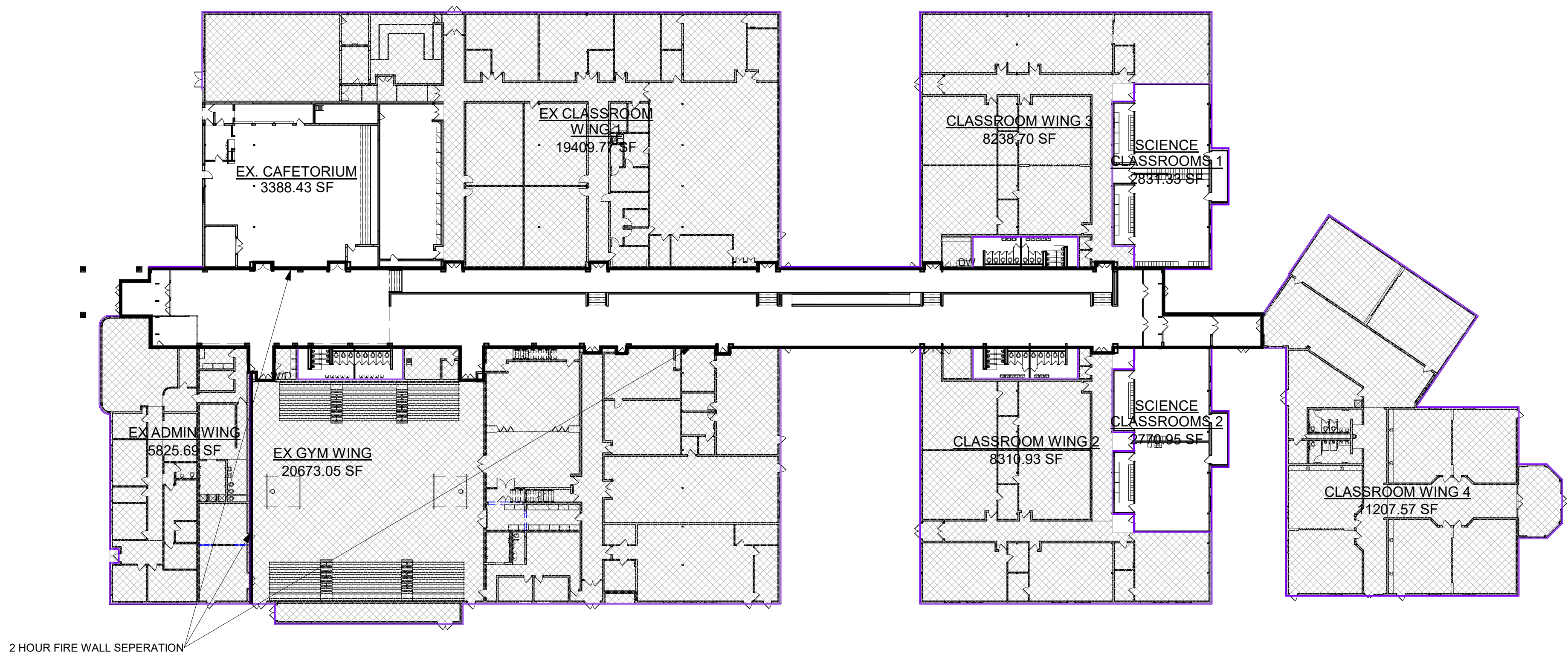
3 LEVEL 1 - EX. FIRE WALL SEPERATION PLAN A0.02 1/32" = 1'-0"
