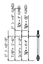
Typ. Anchor Bolts Threaded Rod w/ Double Nut ASTM - F1554 Grade 36
