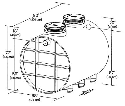
This unit is certified to ASME Al12.14.3 (Type C) and CSA B481.1 and includes an flow control External flow
