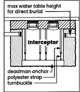
scenarios must be installed with an anchor kit. Models GB-50, GB-75, and GB-250 use model AK1 anchor kit. Model GB-500 uses model AK2 anchor kit for use with deadmen anchors. Models GB-1000, GGI-750 and GGI-1500 use model AK3 anchor kit for use with deadmen anchors.
