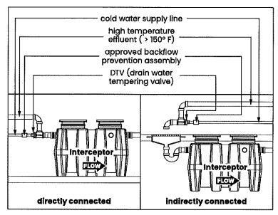
If water is entering the interceptor at excessive temperature (over 150° F), a drain water tempering valve (DTV) and approved backflow prevention assembly must be installed. Most state and local plumbing codes prohibit water above 150° F being discharged into the sanitary sewer. Water above 150° F will weaken or deform PVC Schedule 40 pipe, poly drainage fixtures like interceptors and erode the coating of cast iron (leading to eventual failure).
