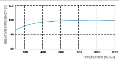
Typical module performance under low irradiance conditions in comparison to STC conditions (25 °C, 1000 W/m²)
