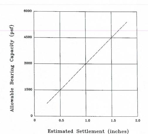
Note: These values are based on footing widths of 1 to 4 feet. If the footing width is to be greater than 4 feet in width, then we should be notified to re-evaluate these recommendations.
