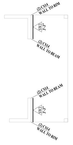
TRUSS MANUFACTURER PROVIDE DRAG TRUSS ALIGNED WITH SHEAR WALLS CAPABLE OF TRANSFERRING 1600 LBS FROM
