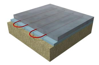
Note: Tube depth is measured from top of embedded layer to the centerline of the tubing.
