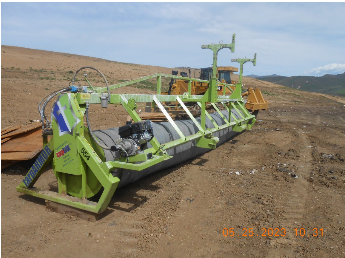
Photo 16: Tarp system used for alternative daily cover at the working face of the landfill
