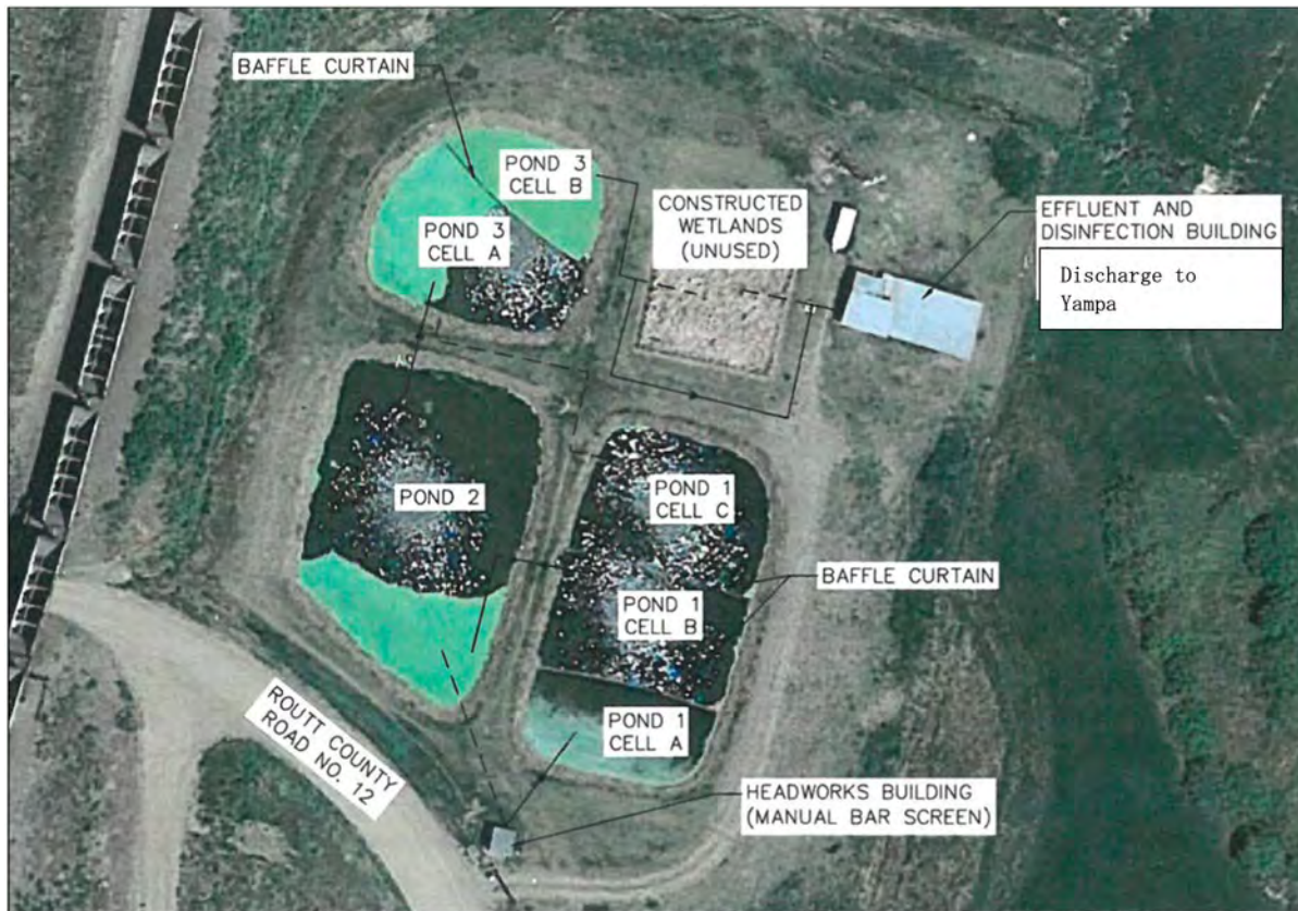
Figure 9: Existing Treatment Plant Schematic
