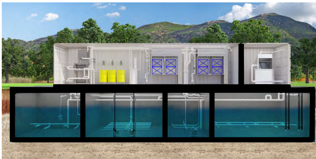
Figure 22: Cross-section View of Newterra Containerized MBR System
