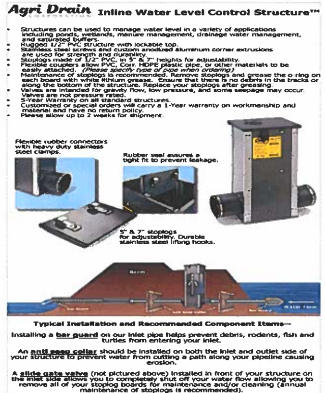
Figure 4-4: Agri-Drain Description and Component Details.
