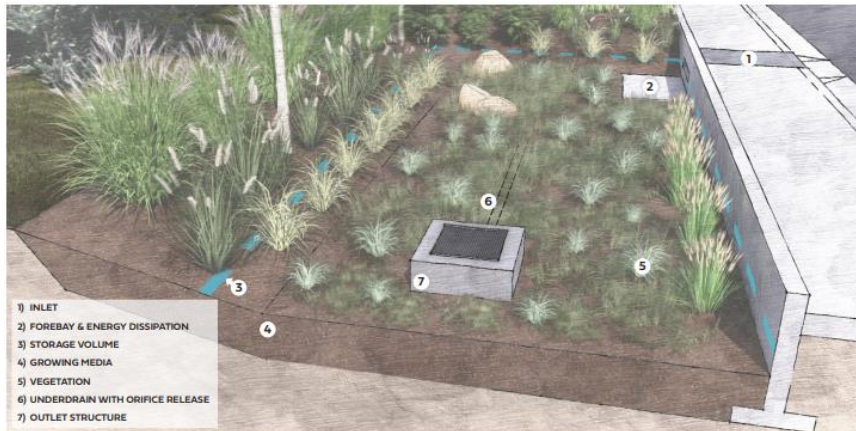
Figure BR-1. Bioretention System Components
