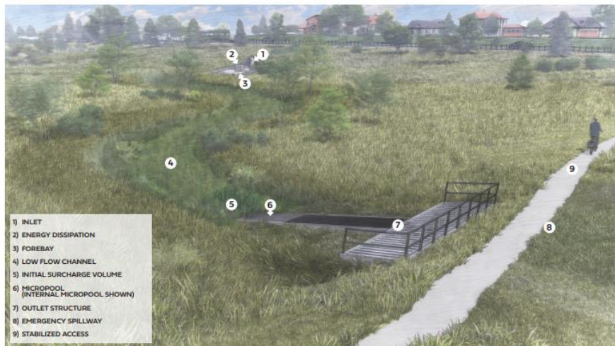
Figure EDB-1. Extended Detention Basin Components
