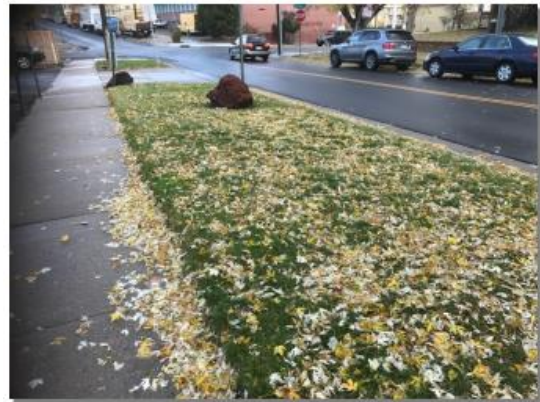
Photograph 3-1. Separate Pervious Area (SPA) is permeable but does not receive runoff from impervious areas, such as the tree lawn in this photo. The drive and street are examples of DCIA.
