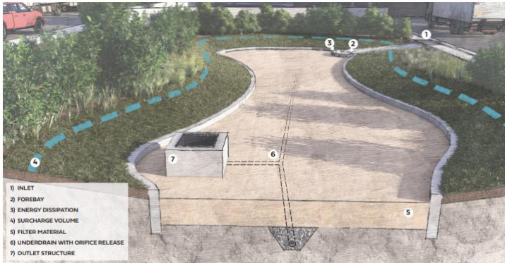
Figure SF-1. Sand Filter Components
