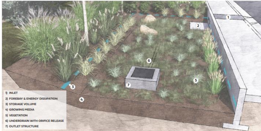
Figure BR-1. Bioretention System Components
