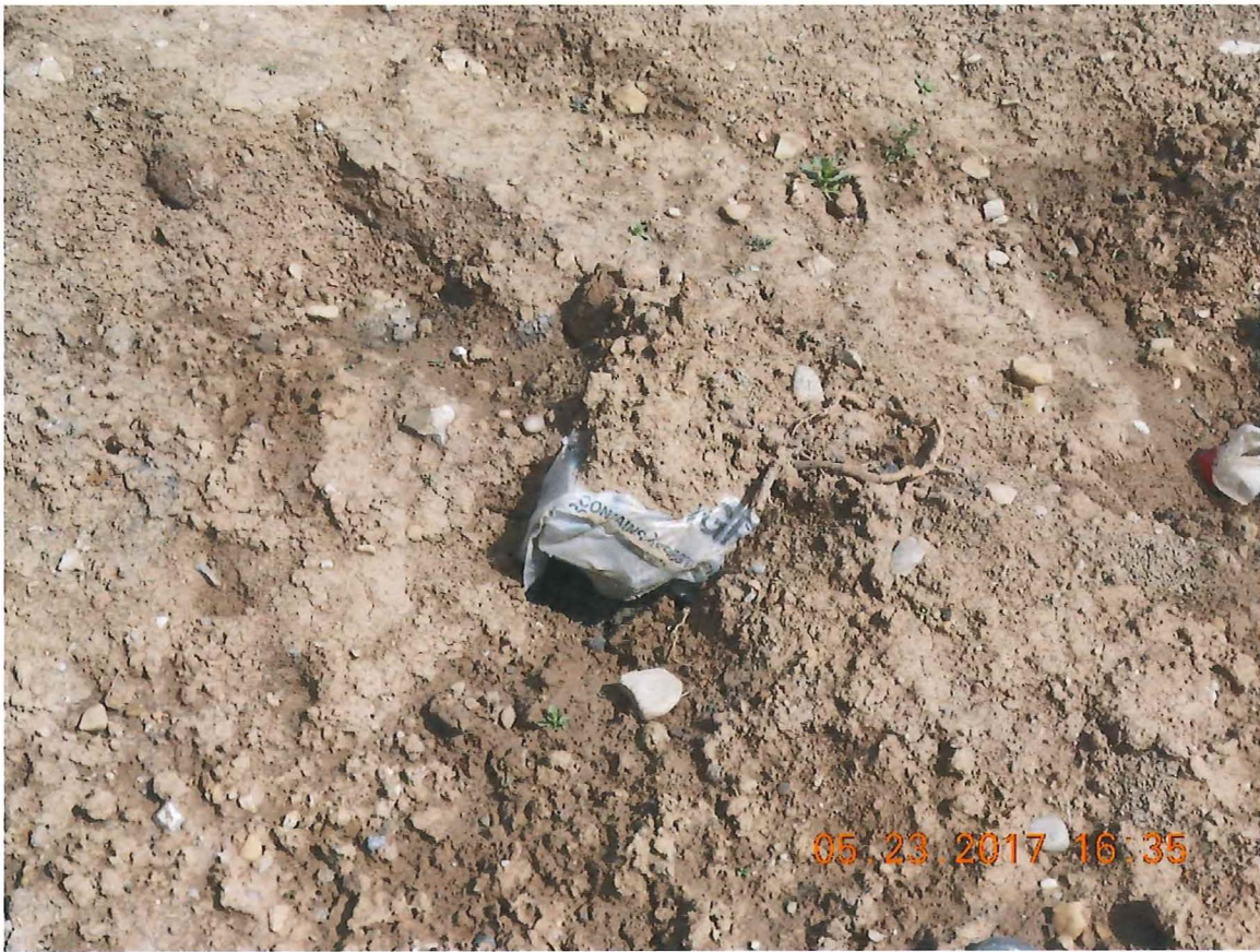
Photo 45: Uncovered asbestos waste
