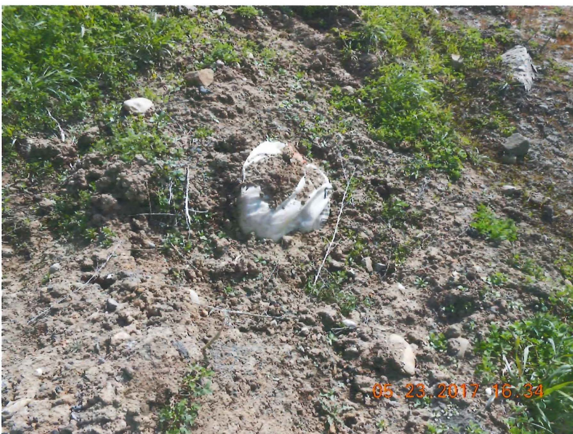
Photo 44: Uncovered asbestos waste
