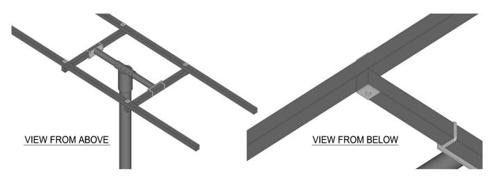
Place longitudinals on top of cross pieces and bolt with square washers top and bottom.
