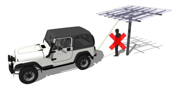
**DO NOT** stand between post and lower side of the array while seasonally adjusting tilt angle.
