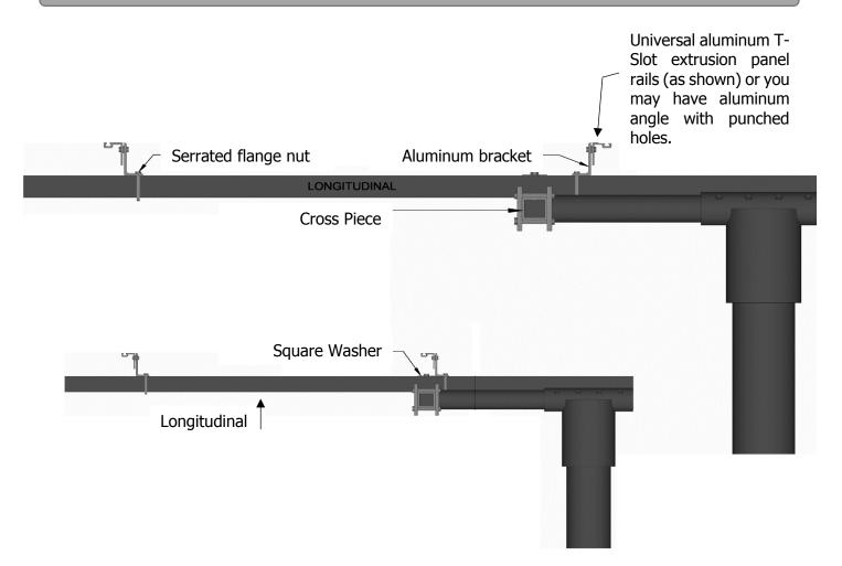
Bracket orientation in most installations is generally opposed to one another as in top picture. It may be necessary to have brackets facing in same direction as in bottom picture, if panel size is such that you need to do this to maintain a <sup>1</sup>/<sub>4</sub>" gap between panel ends on centerline.
