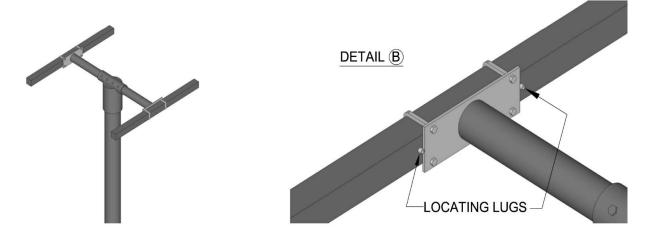
Slide cross pieces into U-bolts. Make sure locating lugs on cross pieces are facing in. See Detail B of locating lugs. Tighten U-bolts.
