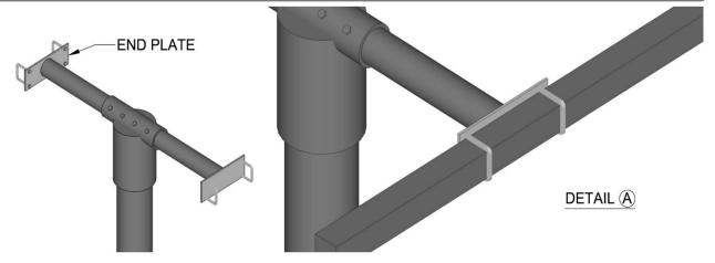
Finger tighten U-bolts (bag #4) onto "Tee" end plates. Place entire "Tee" assembly on top of pipe. Tighten both set bolts and the four bolts on the top of the "Tee". The U-bolts are shown in Detail A.
