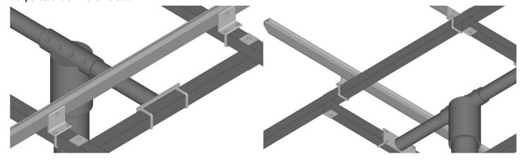
See detail on page 7 for rail/angle bracket assembly. Attach aluminum rails as shown. If rail ends are marked "TOP", align them to the same end.
