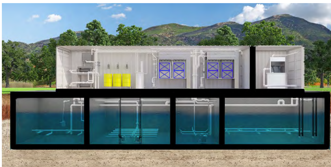
Figure 22: Cross-section View of Newterra Containerized MBR System
